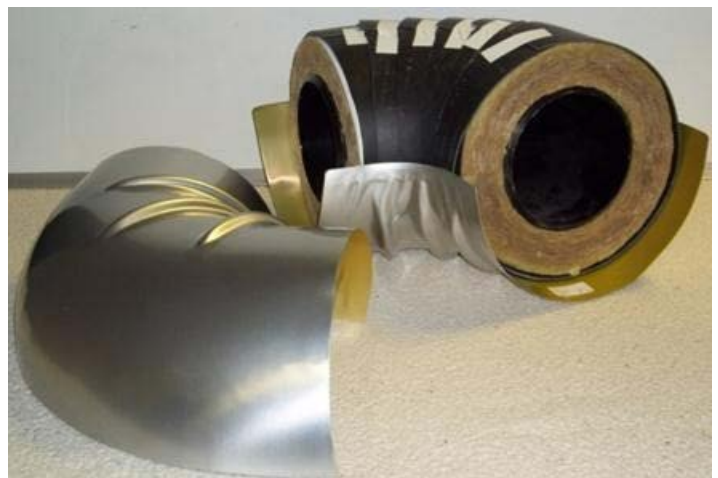
FIGURE 9: Two piece pressed metal elbow shown being applied around mass loaded vinyl on elbow and secured with banding.
