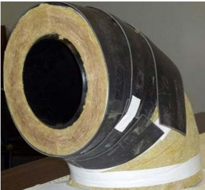
FIGURE 7: Mass loaded vinyl mitered sections (gores) placed around insulation with longitudinal joint at about 3 o'clock and with required \geq 1.3 cm ( \geq \frac{1}{2} inch) longitudinal overlap. Also shown is overlap at circumferential joint which is required to be a maximum of 1.3 cm ( \frac{1}{2} inch).
