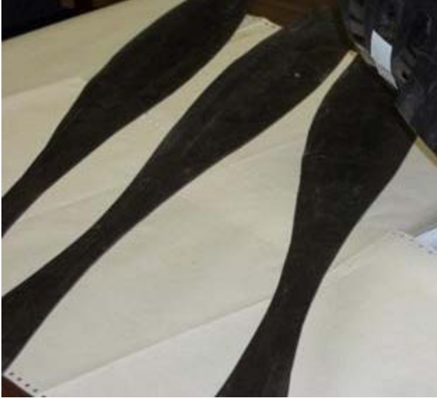
FIGURE 6: Mass loaded vinyl mitered sections (gores) cut to shape and length to fit around insulation with \geq 1.3 cm ( \geq \frac{1}{2} inch) longitudinal overlap.
