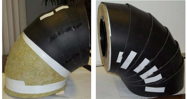
FIGURE 8: Tape or staples are used to lightly secure mass loaded vinyl mitered sections (gores) in place at both longitudinal and circumferential joints.
