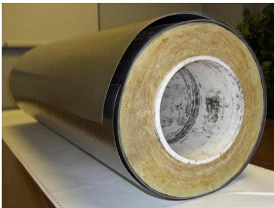
FIGURE 1: Muffl-Jac jacketing with required \geq 5.1 cm (2") longitudinal overlap. Joint located at 3 o'clock position with joint opening pointed downward to naturally shed water.
