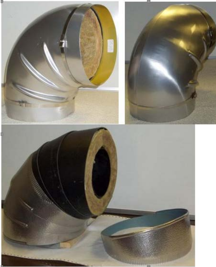
FIGURE 10: Mitered metal jacket sections (gores) applied using standard bead/crimp at circumferential joint and ≥1.3 cm (½ inch) overlap at longitudinal joint which is located at about 3 o'clock.
