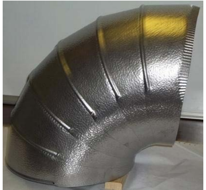
FIGURE 11: Finished mitered metal jacket sections (gores) applied to elbow over mass loaded vinyl.
