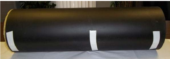
FIGURE 4 – Mass loaded vinyl secured lightly with tape.
