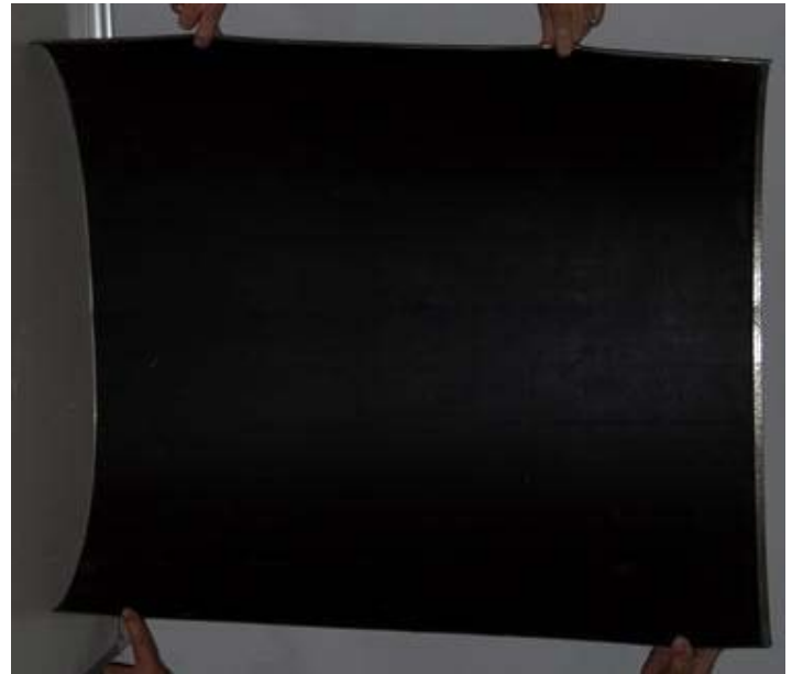
FIGURE 5 – Muffl-Jac jacketing cut to fit around first layer of mass loaded vinyl and yield the required \geq 5.1 cm (2") longitudinal overlap.
