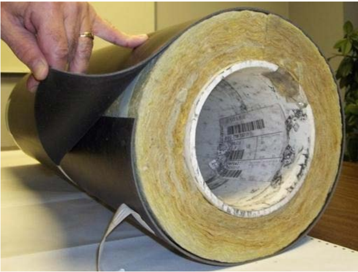
FIGURE 3: Mass loaded vinyl (MLV) with required \geq 5.1 cm (2") longitudinal overlap. Joint located at 3 o'clock position with joint opening pointed downward to naturally shed water.
